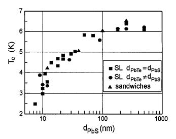
FIG. 1. Transition temperature as a function of  $d_{PbS}$  for PbTe/PbS layered samples.
