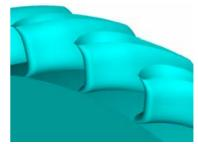
Figure 7. Optimized guide blade rim for a/l=0.22
