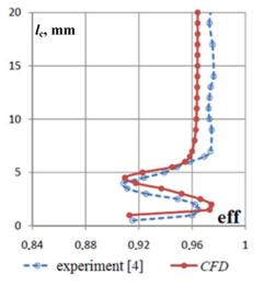
Figure 1. Efficiency distribution along blade height
