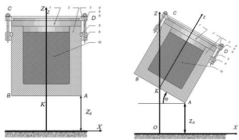
Fig. 2 The cases at impact: 1) Vertical impact on the base, 2) Oblique impact on bottom corner at angle of 30° from the horizontal
