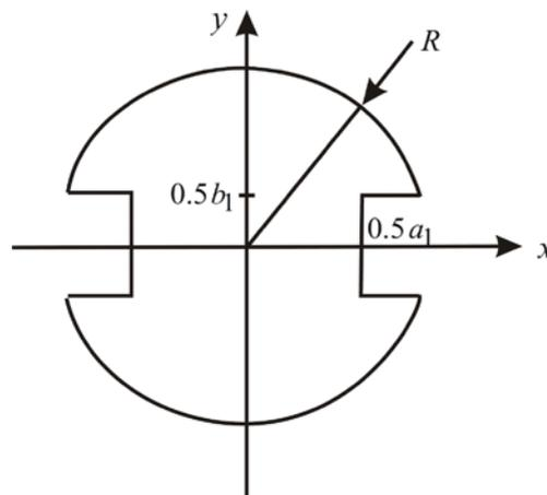
Fig.1 Circular plate with two cutouts
