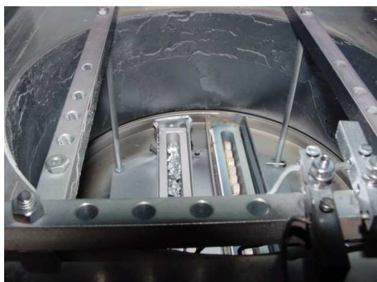
Fig. 1 Vacuum chamber for thermal vacuum evaporation of CdTe and CdS films.
