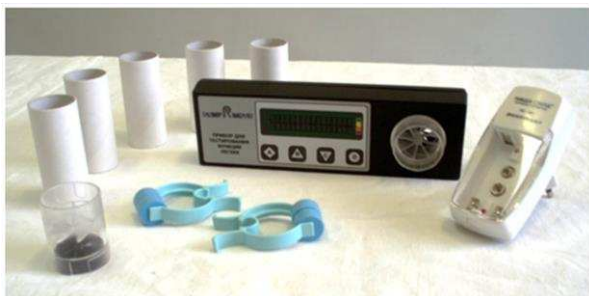
Components of digital portable spirometer DS-14/1
