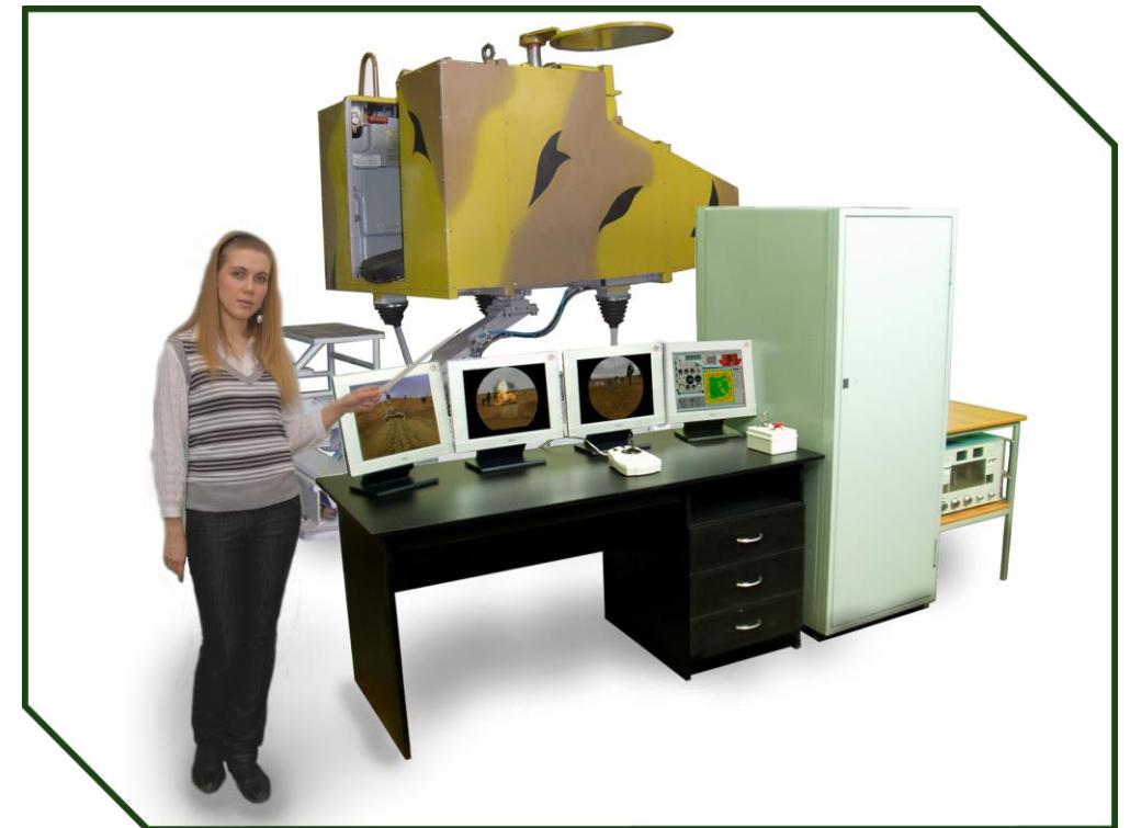
Computer Training System for Armored Vehicles (Driver Cockpit, Processing Server and Trainer Workpost)
