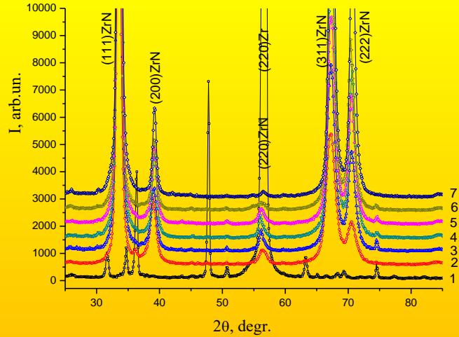
Research the multilayer compositions of single- and multicomponent nitrides of transition metals (including high-entropy alloys (TiAlHfVNb)<sub>N</sub>, (TiAlHfVNb)<sub>N</sub>, (TiAlHfVNbtTa)<sub>N</sub>, (FeCoNiNbCrCuV)<sub>N</sub>), (TiAlCrSiNb)<sub>N</sub>, with high and ultrahigh hardness. Structural Engineering of steels surfaces (including the formation of S-phase, etc.) by means of ion nitriding, followed by coating nitride or metal coatings.
